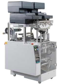
SC-9100H2 with coin fed to both counting head from a SCAN COIN bulk coin lift.
